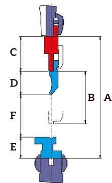
A = distance table/ram | B = stroke | C = net height adapter | D = net height punch | E = net height die | F = net opening
